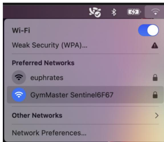
2. After selecting the GymMaster Sentinel Wifi signal enter in the AP password listed on the back of the reader.
